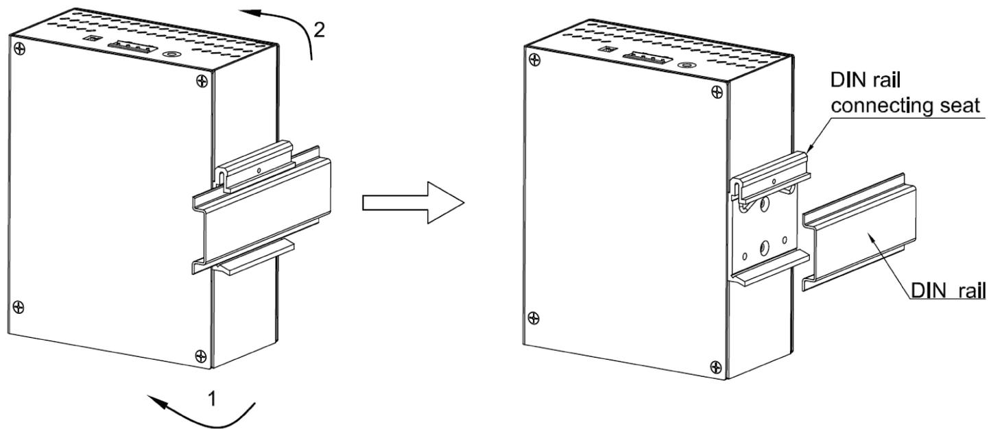
Figure 6 DIN Rail Dismounting
