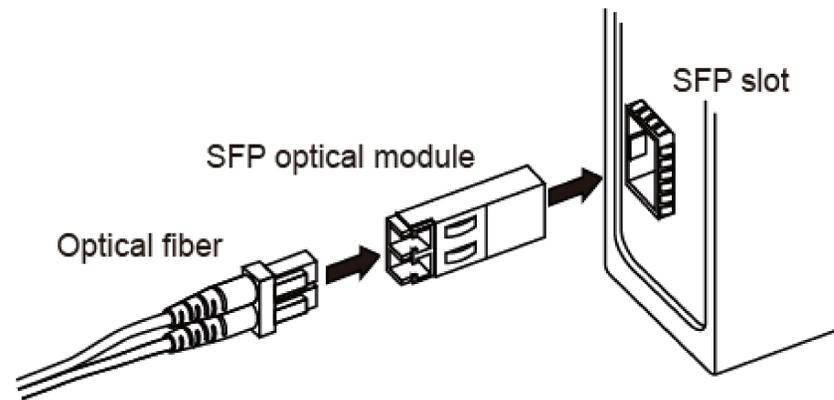
Figure 14 Connecting the SFP Optical Module
