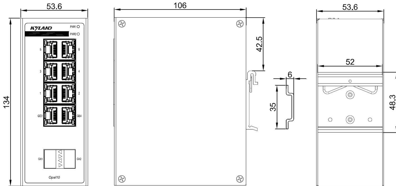
Figure 3 Opal10 Dimensions for DIN-Rail Mounting (unit: mm)
