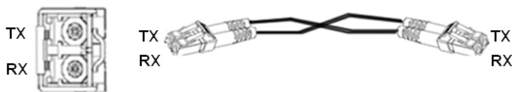
Figure 13 Fiber Connection of an SFP Optical Module
