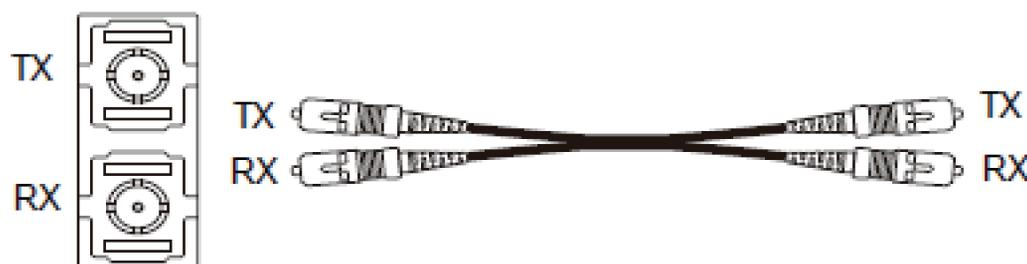
Figure 9 Connection of 100Base-FX Ethernet Port
