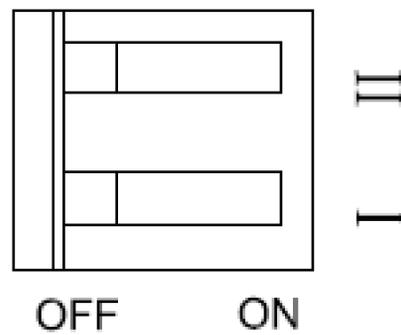
Figure 16 DIP Switches
