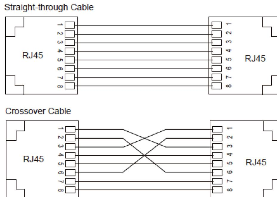
Figure 8 Connection Using Straight-through/Cross-over Cable
