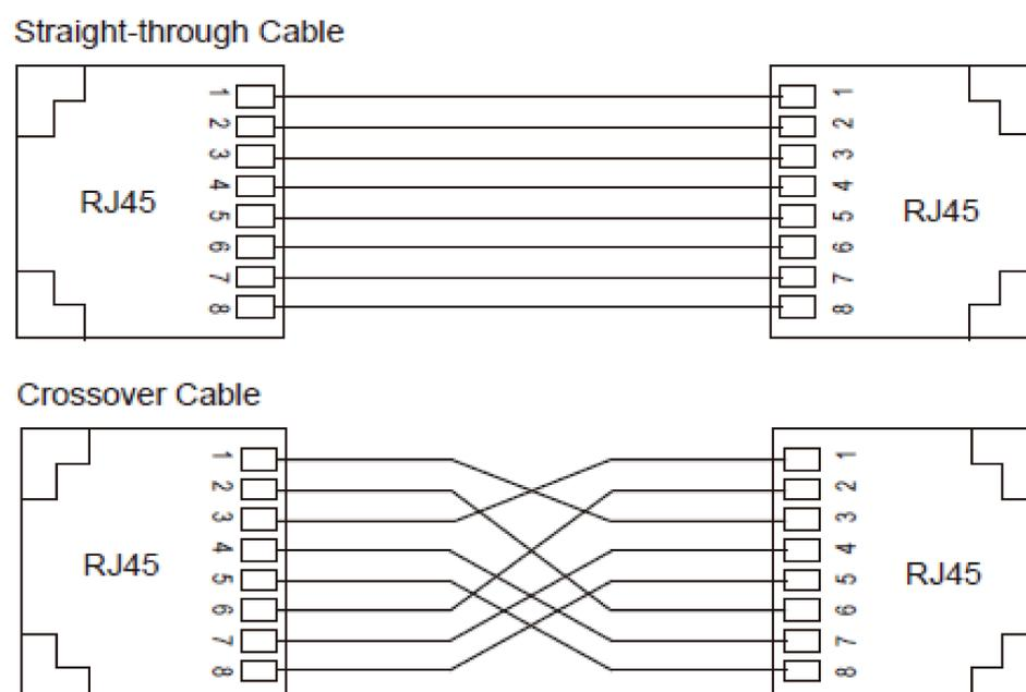
Figure 11 Connection Using Straight-through/Cross-over Cable
