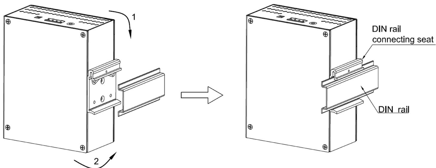
Figure 5 DIN-Rail Mounting
