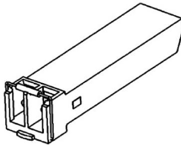
Figure 12 SFP Optical Module
