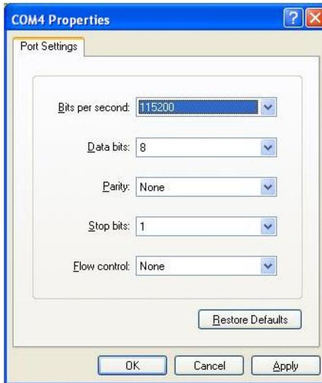
Figure 24 Setting Port Parameters
