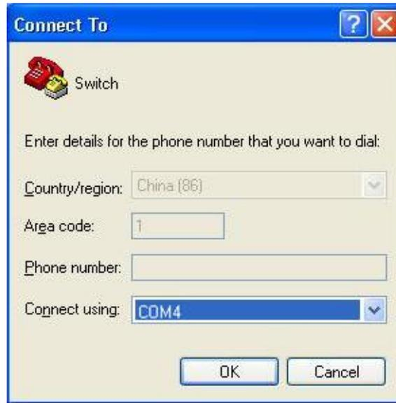
Figure 20 Selecting the Communication Port in Use
