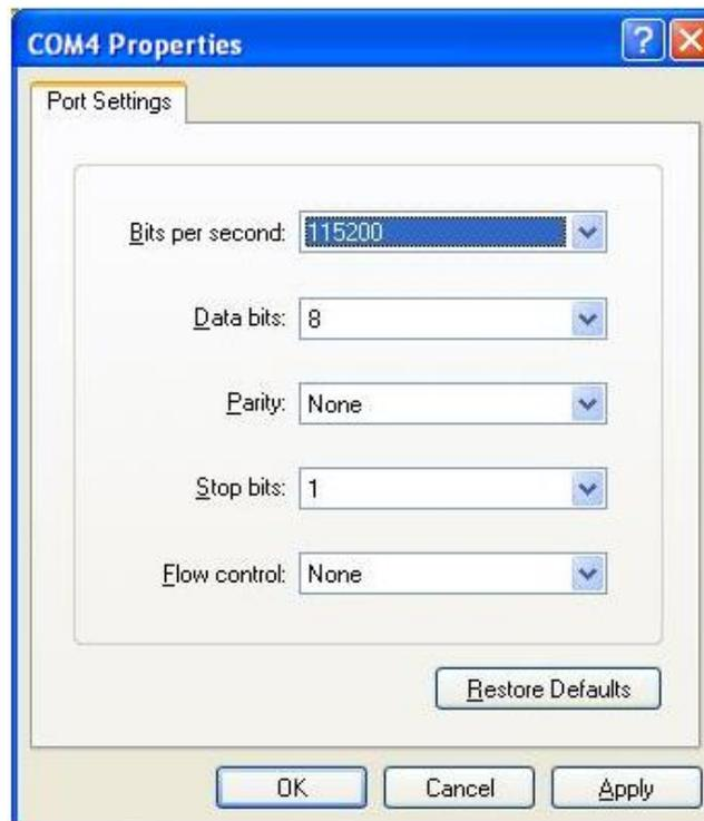
Figure 21 Setting Port Parameters
