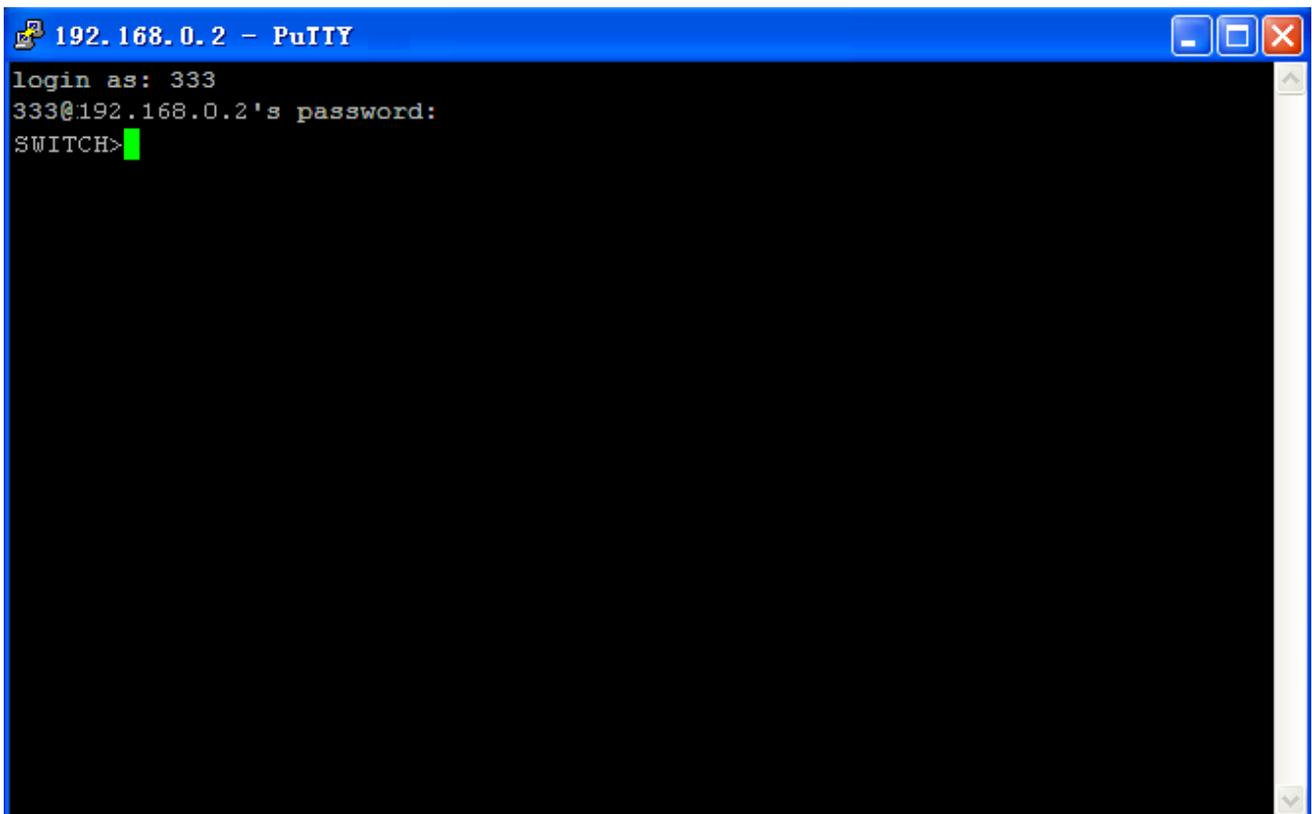
Figure 72 Login Interface of the SSH Password Authentication
