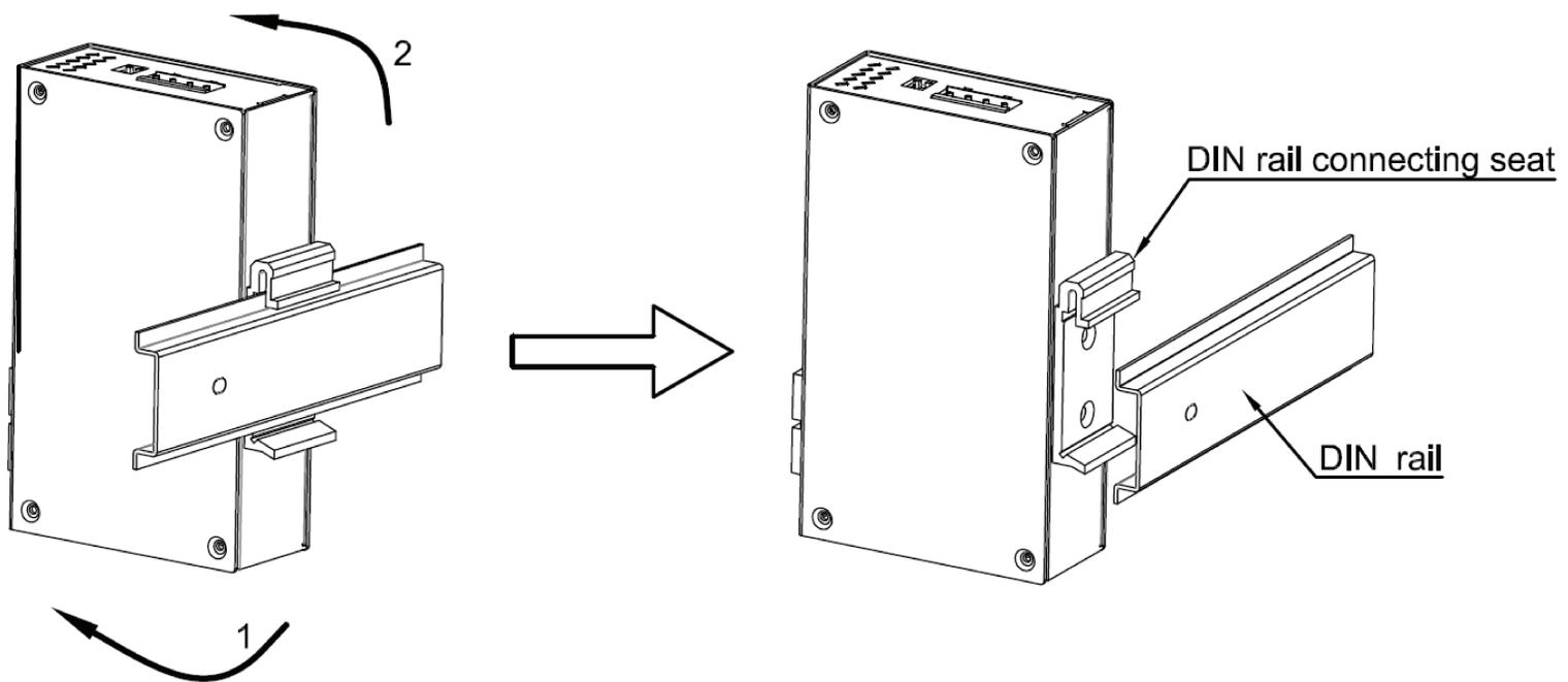
Figure 6 DIN Rail Dismounting
