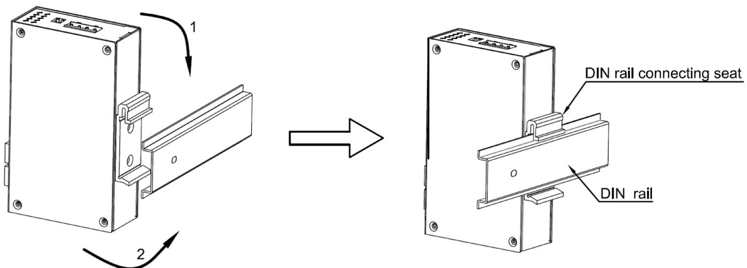
Figure 5 DIN-Rail Mounting
