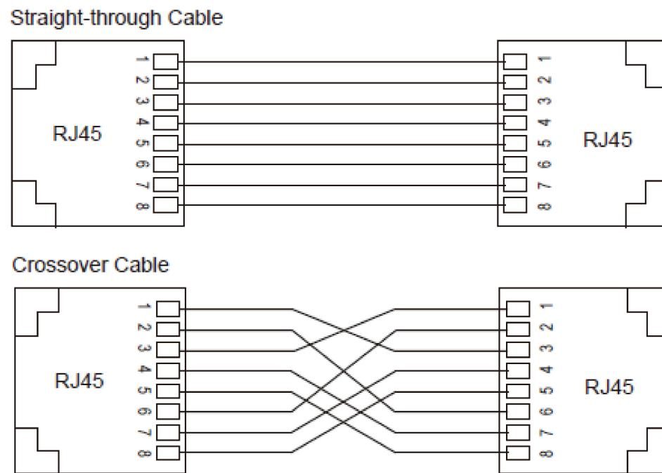
Figure 8 Connection Using Straight-through/Cross-over Cable
