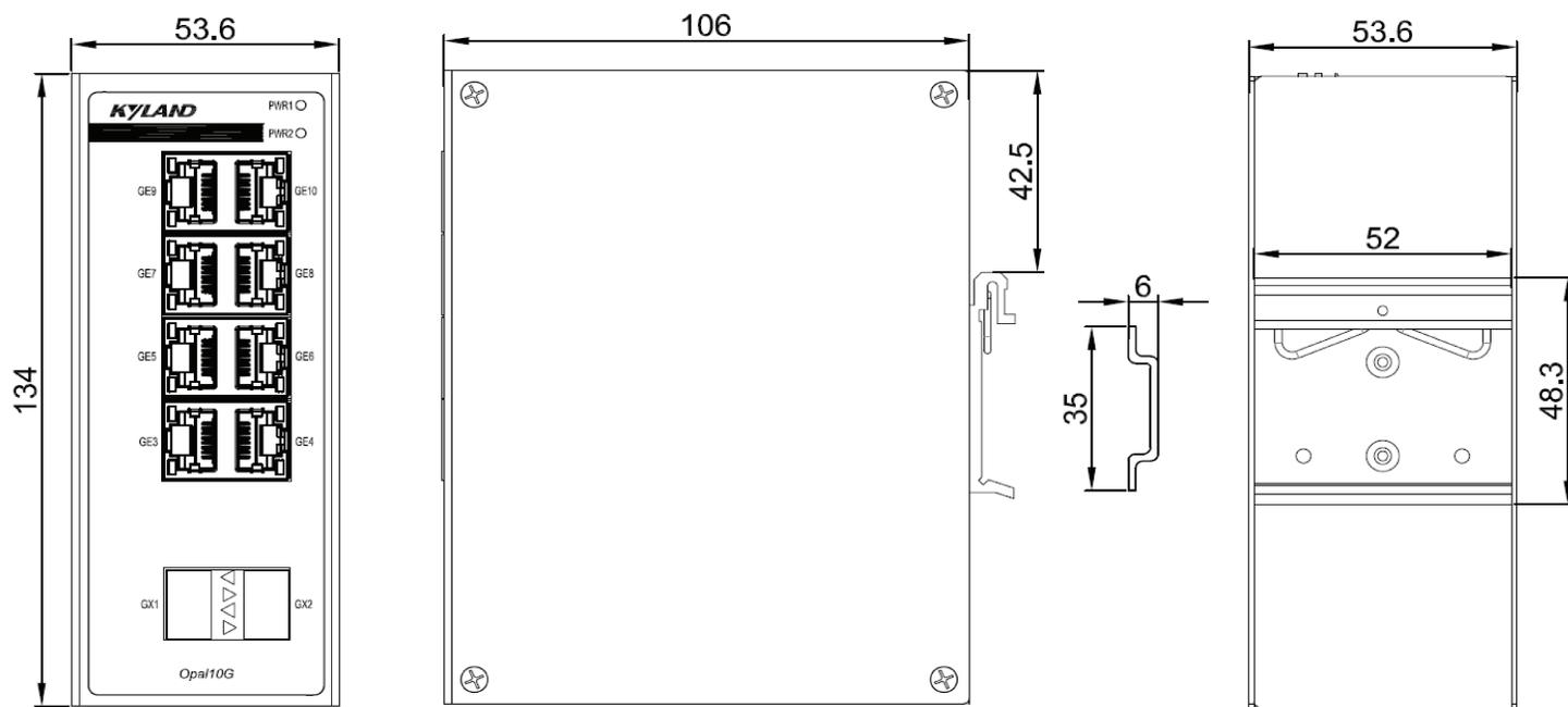
Figure 4 Opal10G Dimensions for DIN-Rail Mounting (unit: mm)
