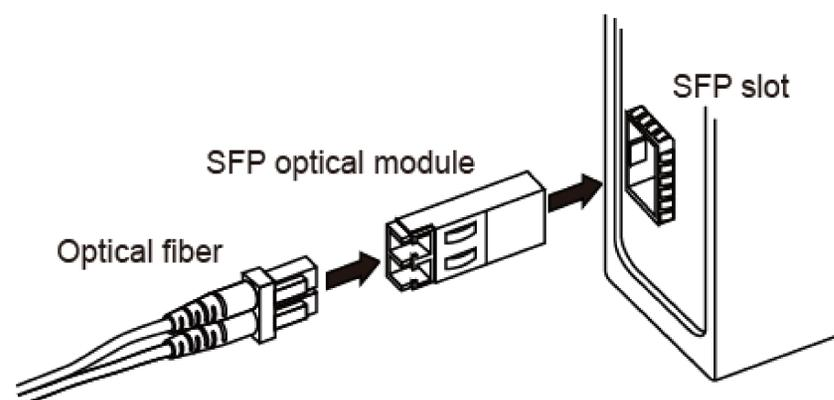
Figure 11 Connecting the SFP Optical Module
