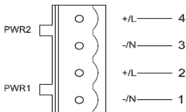
Figure 12 4-Pin 5.08mm-Spacing Plug-in Terminal Block (socket)
