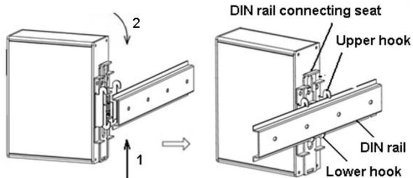
Figure 3 DIN-Rail Mounting
