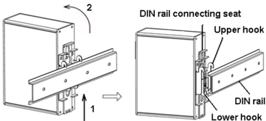
Figure 4 Removing KOM200 from DIN Rail
