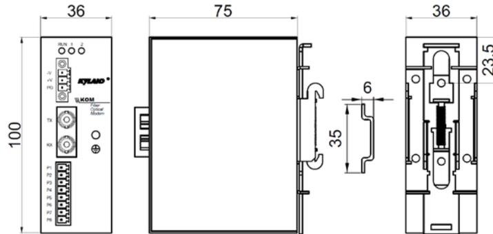
Figure 2 Dimensions for DIN-Rail Mounting (Unit: mm)
