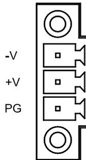
Figure 8 3-Pin 3.81mm-Spacing Plug-in Terminal Block (socket)
