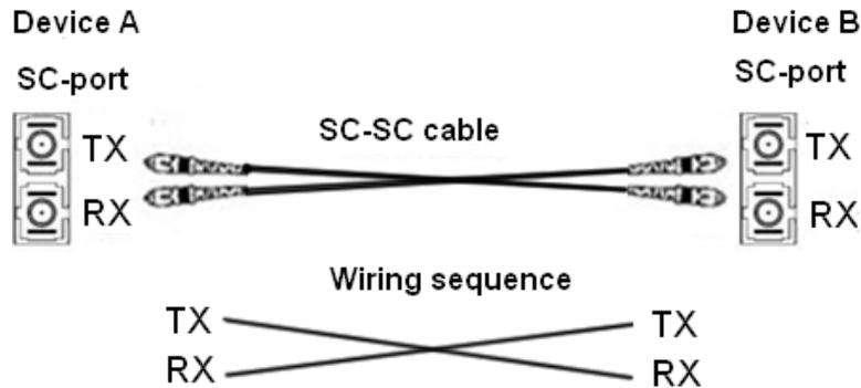
Figure 5 Wiring of Fiber Port
