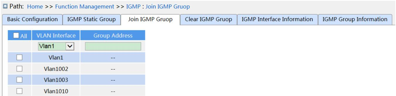
Figure 227 join IGMP Group configuration
