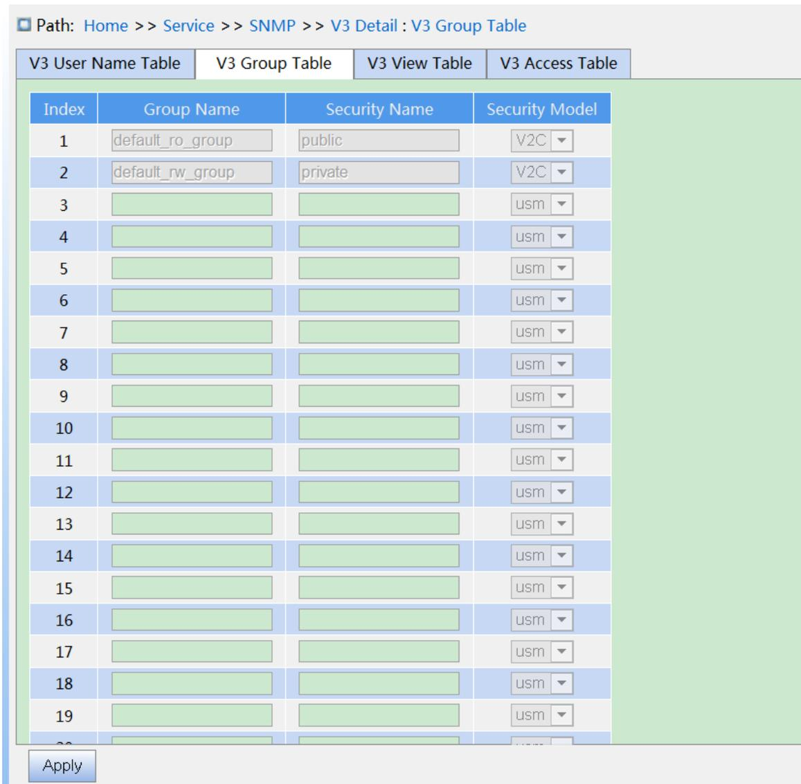
Figure 58 Configure SNMPv3 group table
