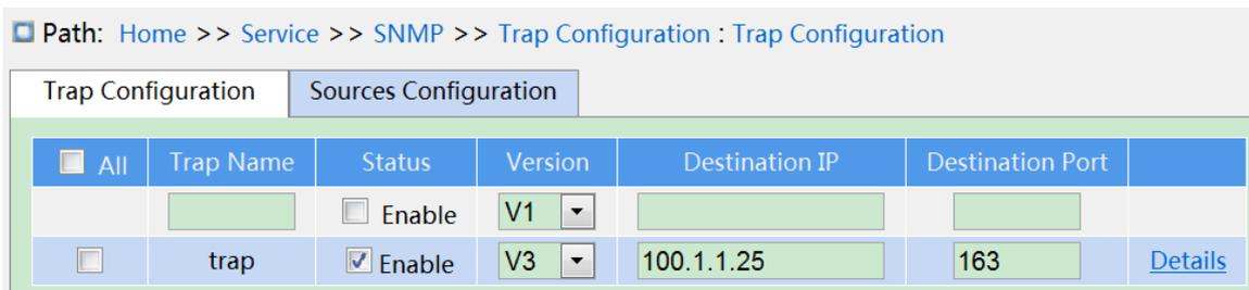
Figure 54 Configure Trap
