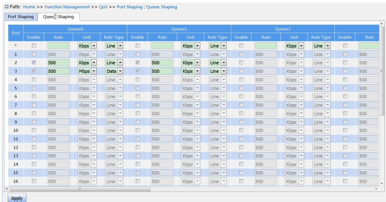
Figure 273 Configure Queue shaping
