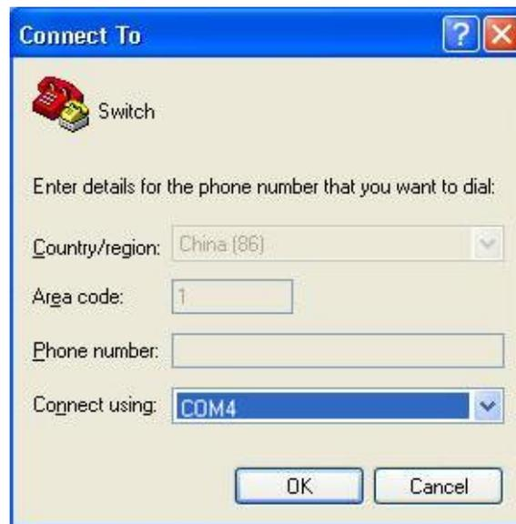
Figure 25 Selecting a Serial Port
