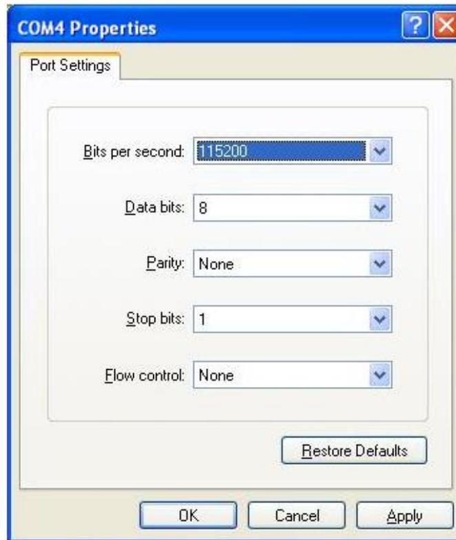
Figure 26 Setting Port Parameters
