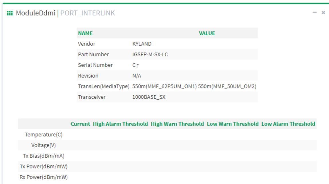
Figure 90 L port optical module information
