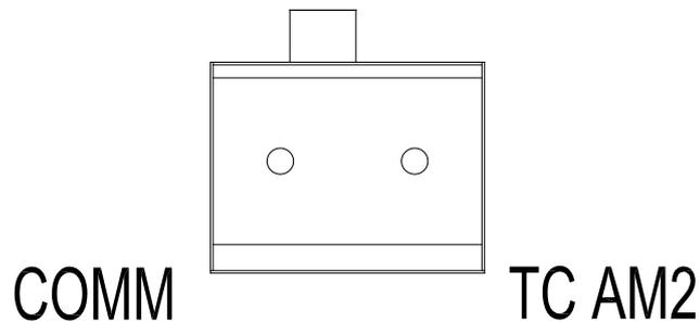
Figure 15 2-pin 5.08mm-spacing Plug-in Terminal Block (Socket)
