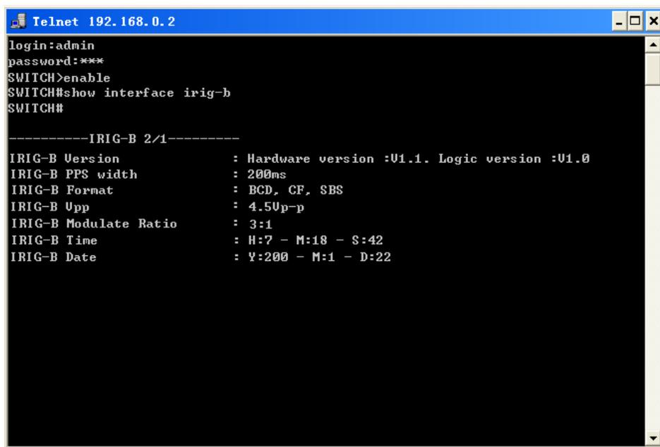
Figure 23 Telnet Configuration Interface
