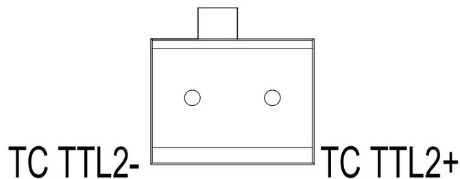
Figure 13 2-Pin 5.08mm-spacing Plug-in Terminal Block (Socket)
