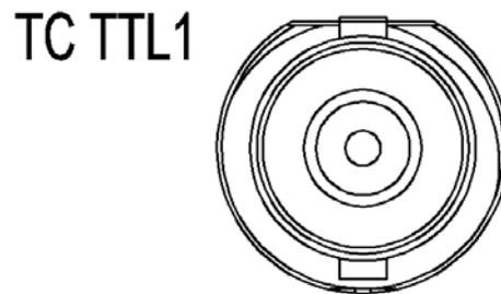
Figure 12 IRIG-B (DC) BNC Connector (female)
