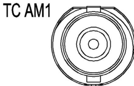
Figure 14 IRIG-B (AC) BNC Connector (female)
