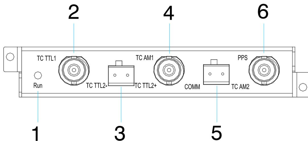
Figure 1 IRIG-B PTP Clock Converter Output Module Panel
