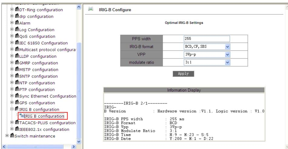
Figure 25 IRIG-B Configuration Interface
