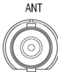
Figure 6 Satellite Signal Input Port
