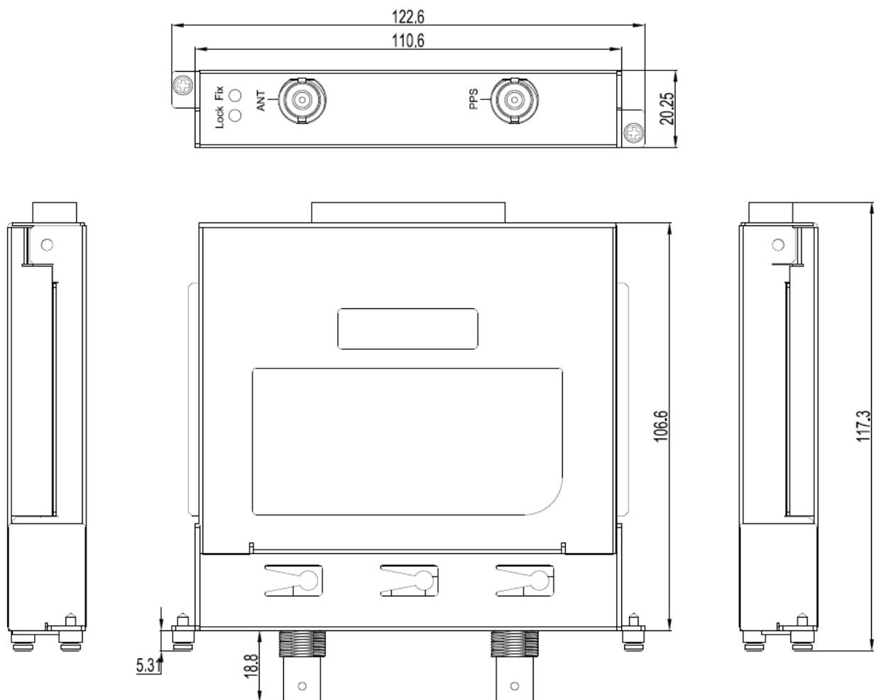
**» Ordering Information****SM6.6-GPS-OI-0.5U:** GPS module, one GPS input, BNC connector; one PPS output, BNC connector
