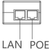
Figure 2 Schematic diagram of the power adapter interface
