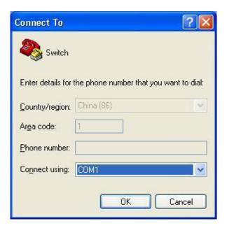
Figure 20 Selecting a Serial Port
