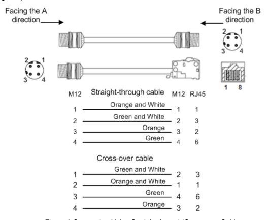
Figure 8 Connection Using Straight-through/Cross-over Cable
