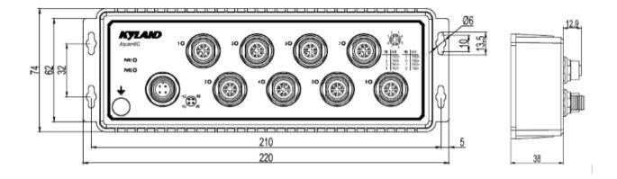
Figure 2 Dimensions (unit: mm)
