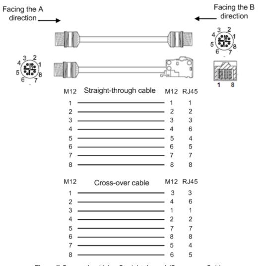
Figure 7 Connection Using Straight-through/Cross-over Cable
