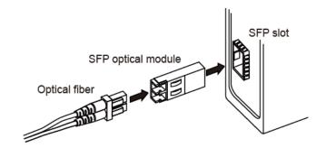
Figure 11 Connecting the SFP Optical Module
