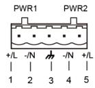
Figure 17 5-Pin 5.08mm-Spacing Plug-in Terminal Block
