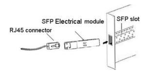
Figure 13 Connecting the SFP Electrical Module
