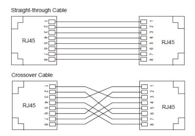
Figure 8 Connection Using Straight-through/Cross-over Cable
