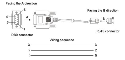
Figure 15 Wiring Sequence of DB9-RJ45 Console Cable
