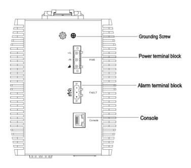
Figure 3 High voltage products Top Panel
