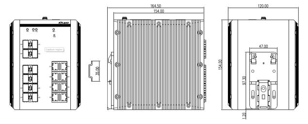
Figure 4 Dimensions for DIN-Rail Mounting (unit: mm)
