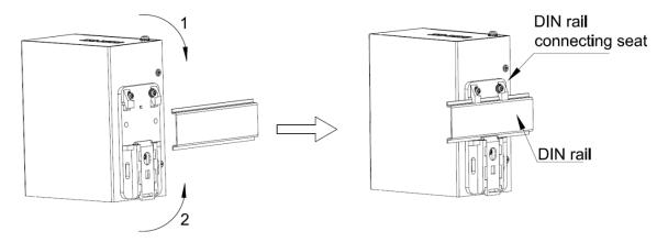
Figure 5 DIN-Rail 2 Mounting
