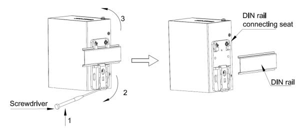
Figure 6 DIN-Rail 2 Dismounting
