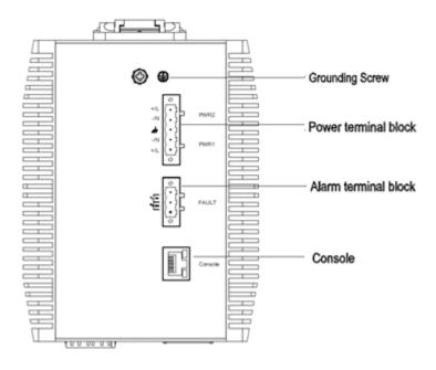
Figure 2 Low voltage products Top Panel
