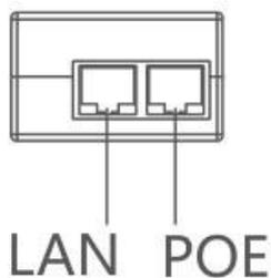
Schematic diagram of the power adapter interface
