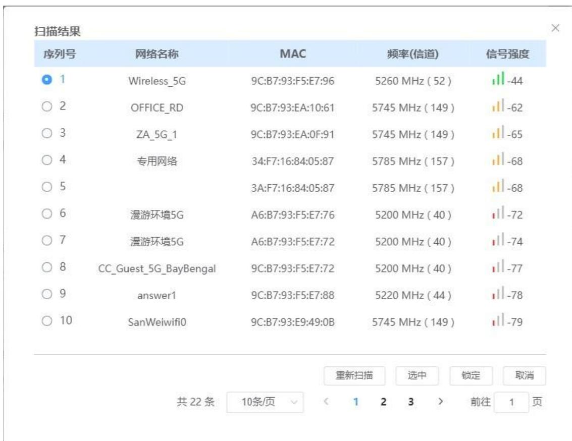
Figure 42 Scanning signal
