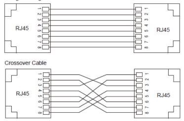
Figure 6 Connection Using Straight-through/Cross-over Cable
