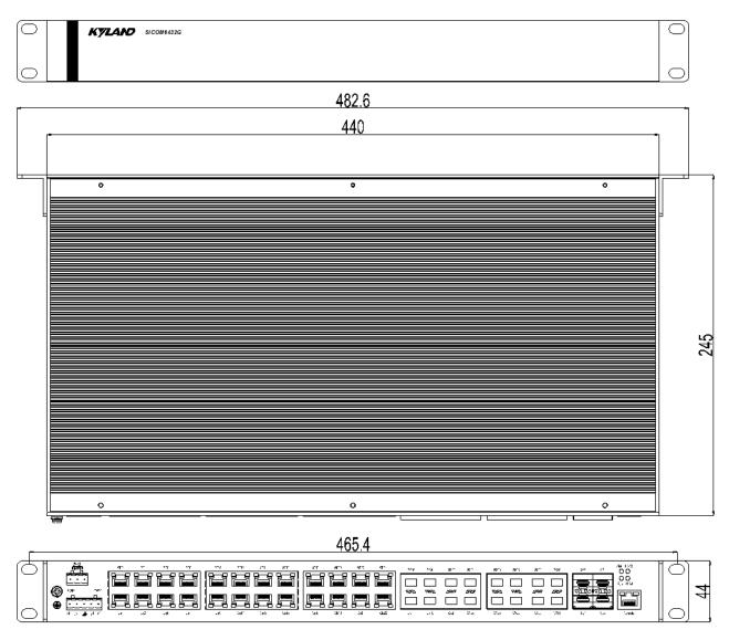
Figure 2 SICOM6432G&3432G Dimensions (unit: mm)
