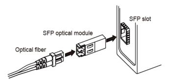
Figure 9 Connecting the SFP Optical Module
