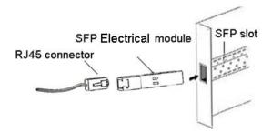
Figure 11 Connecting the SFP Electrical Module
