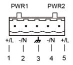
Figure 14 5-Pin 5.08mm-Spacing Plug-in Terminal Block
