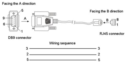
Figure 13 Wiring Sequence of DB9-RJ45 Console Cable
