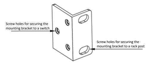
Figure 3 Mounting Bracket
