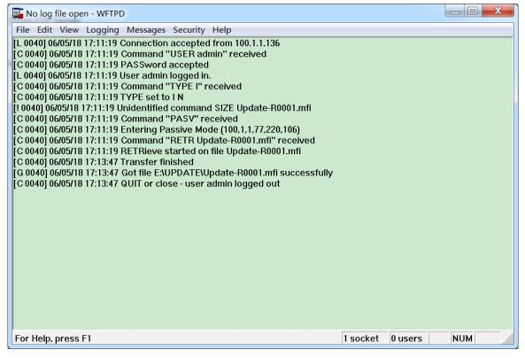
Figure 33 Normal Communication between FTP Server and Switch
