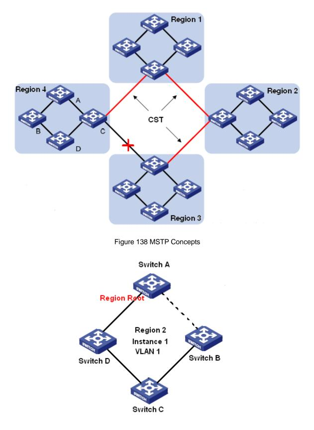
Figure 139 VLAN 1 Mapping to Instance 1
