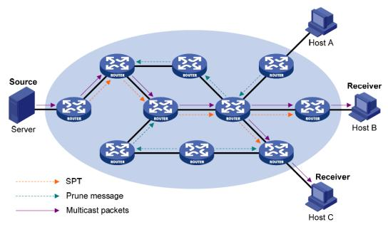
Figure 222 Schematic diagram for building SPT in PIM-DM
