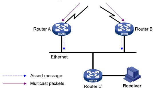
Figure 213 Assert mechanism diagram
