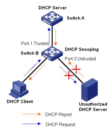
Figure 190 DHCP Snooping Typical Configuration Example
