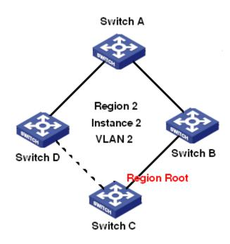
Figure 140 VLAN2 Mapping to Instance 2
