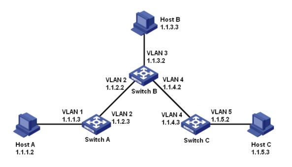
Figure 233 Example for Configuring Static Routes
