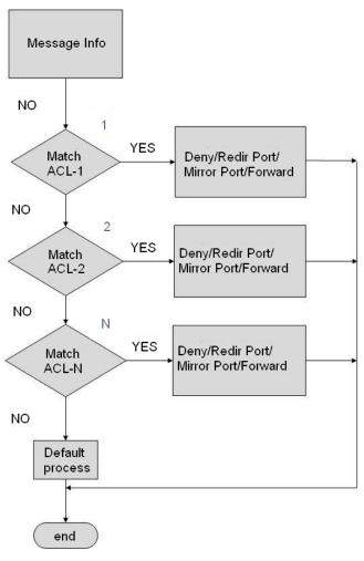
Figure 156 ACL Processing Flowchart
