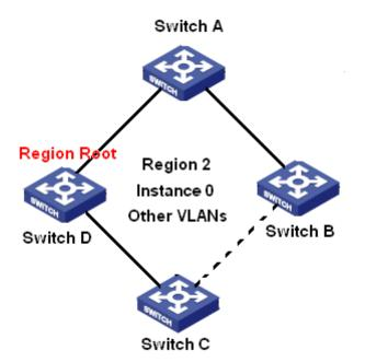
Figure 141 Other VLAN Mapping to Instance 0
