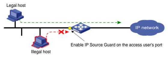
Figure 292 IP Source Guard function diagram
