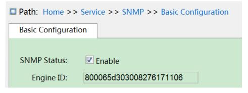
Figure 47 Enable SNMP
