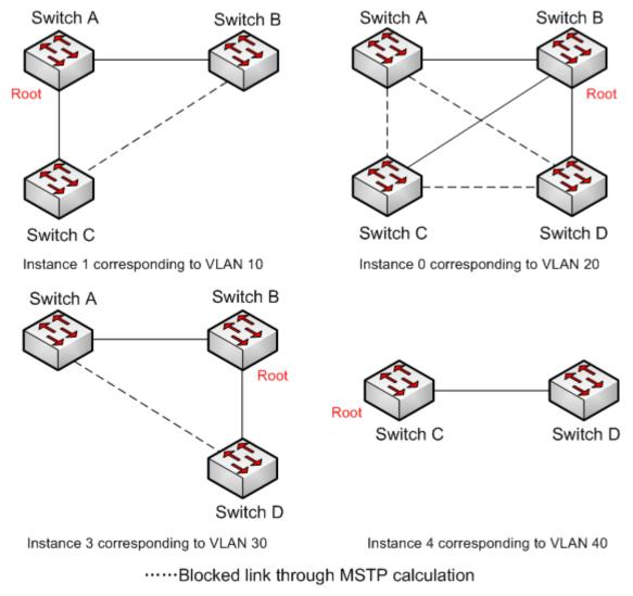
Figure 151 Spanning Tree Instance of each VLAN
