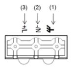
Figure 22 5-Pin 5.08mm-Spacing Plug-in Terminal Block (socket)
