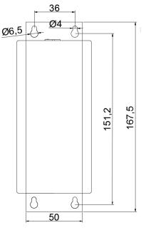
Figure 5 Dimensions for DIN-Rail Mounting (unit: mm)
