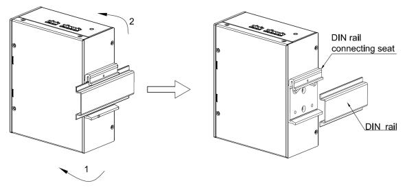
Figure 7 DIN-Rail 1 Dismounting
