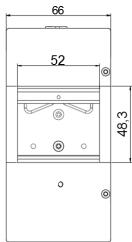
Figure 4 Dimensions for DIN-Rail Mounting (unit: mm)
