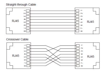
Figure 13 Connection Using Straight-through/Cross-over Cable
