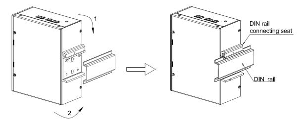
Figure 6 DIN-Rail 1 Mounting
