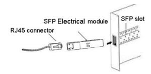
Figure 18 Connecting the SFP Electrical Module
