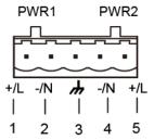
Figure 21 5-Pin 5.08mm-Spacing Plug-in Terminal Block (socket)
