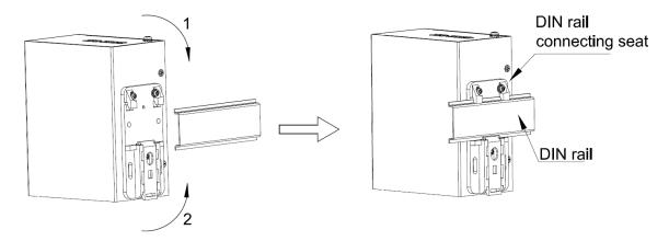
Figure 8 DIN-Rail 2 Mounting
