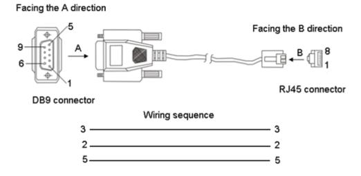
Figure 20 Wiring Sequence of DB9-RJ45 Console Cable
