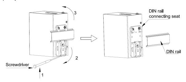
Figure 9 DIN-Rail 2 Dismounting
