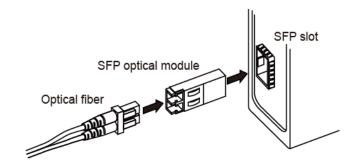
Figure 16 Connecting the SFP Optical Module
