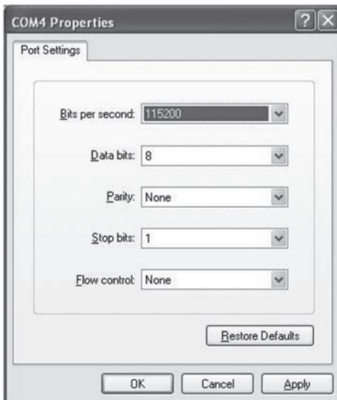
Figure 16 Setting Port Parameters
