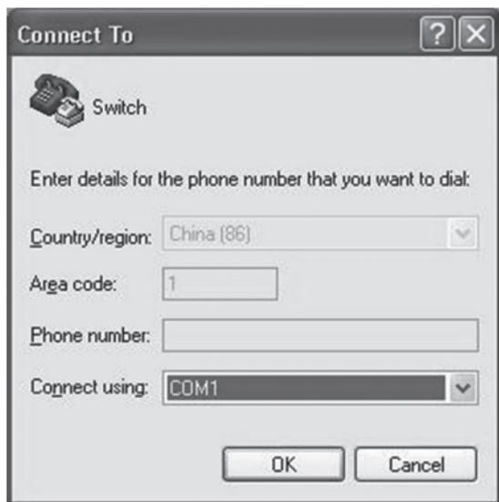
Figure 15 Selecting a Serial Port
