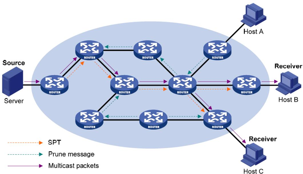
Figure 226 Schematic diagram for building SPT in PIM-DM
