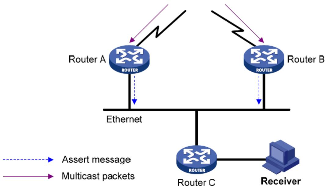
Figure 217 Assert mechanism diagram
