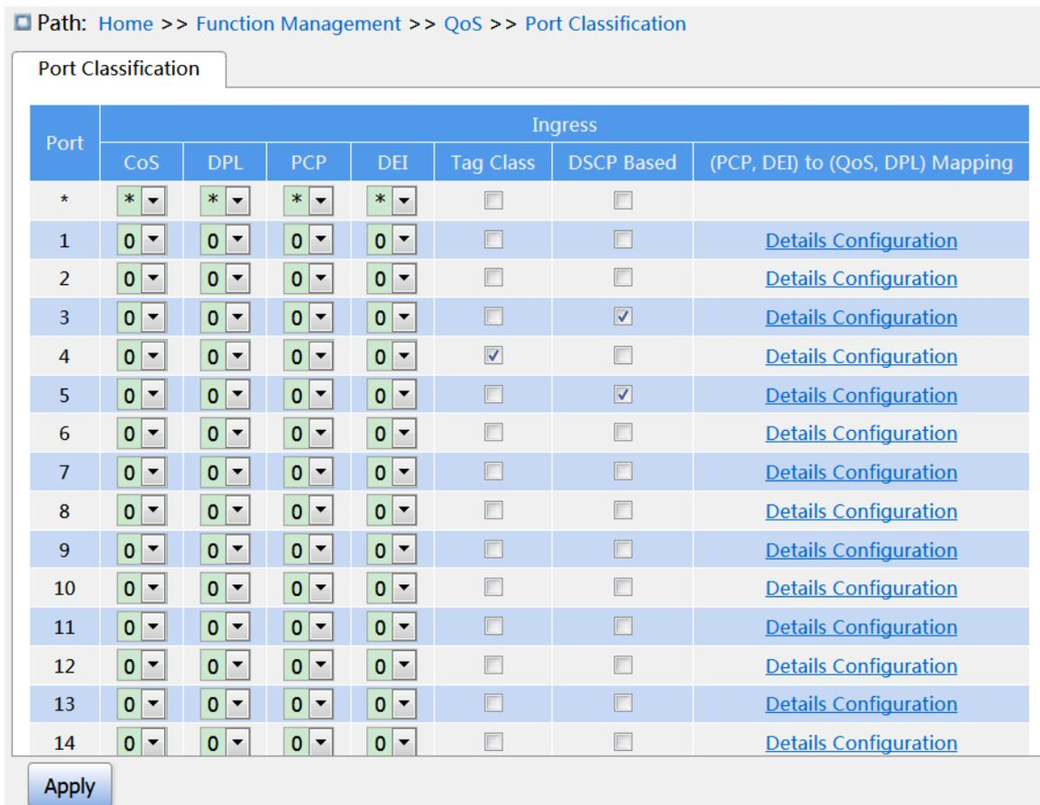
Figure 262 Enable queue mapping mode based on DSCP
