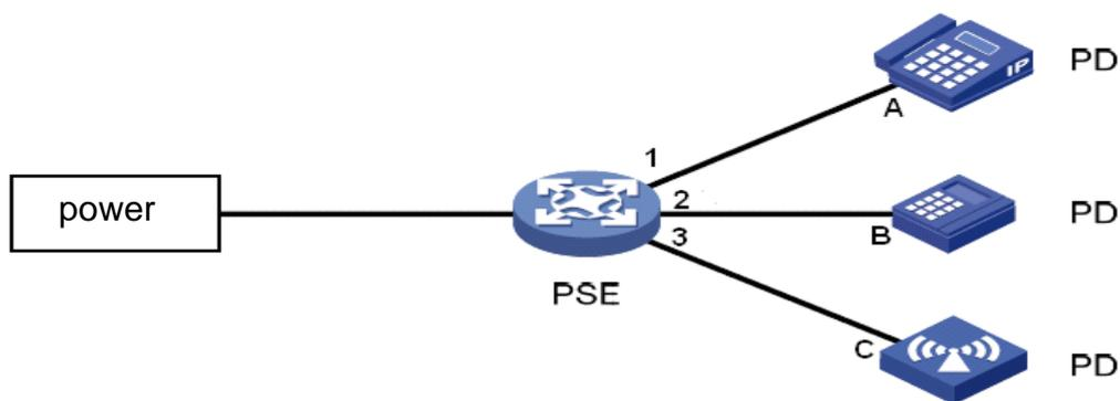
Figure 169 POE power supply system
