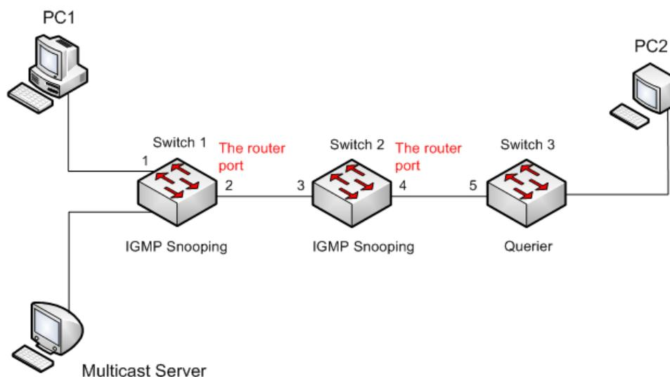
Figure 179 IGMP Snooping Application Example
