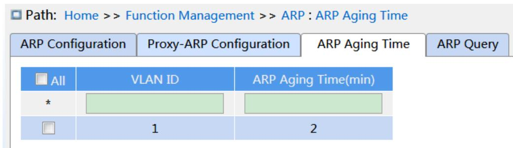
Figure 154 ARP Aging Time Configuration
