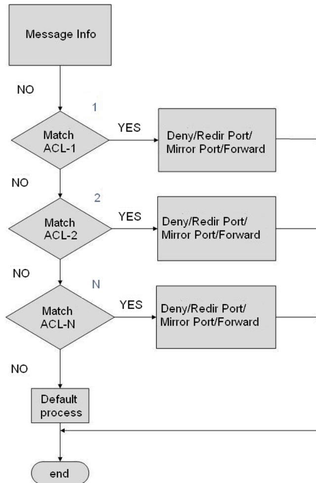
Figure 156 ACL Processing Flowchart
