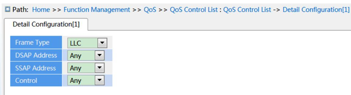
Figure 269 Configure LLC frame parameters
