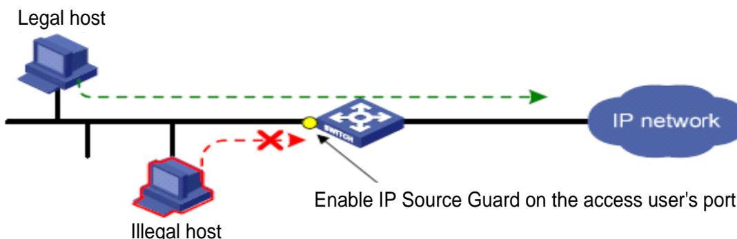
Figure 332 IP Source Guard function diagram
