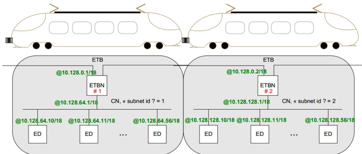
Figure 284 IP address assignment example diagram
