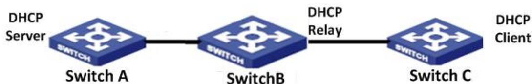
Figure 337 DHCP typical configuration example
