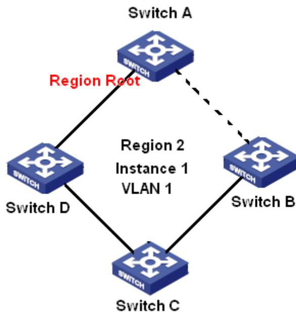
Figure 139 VLAN 1 Mapping to Instance 1
