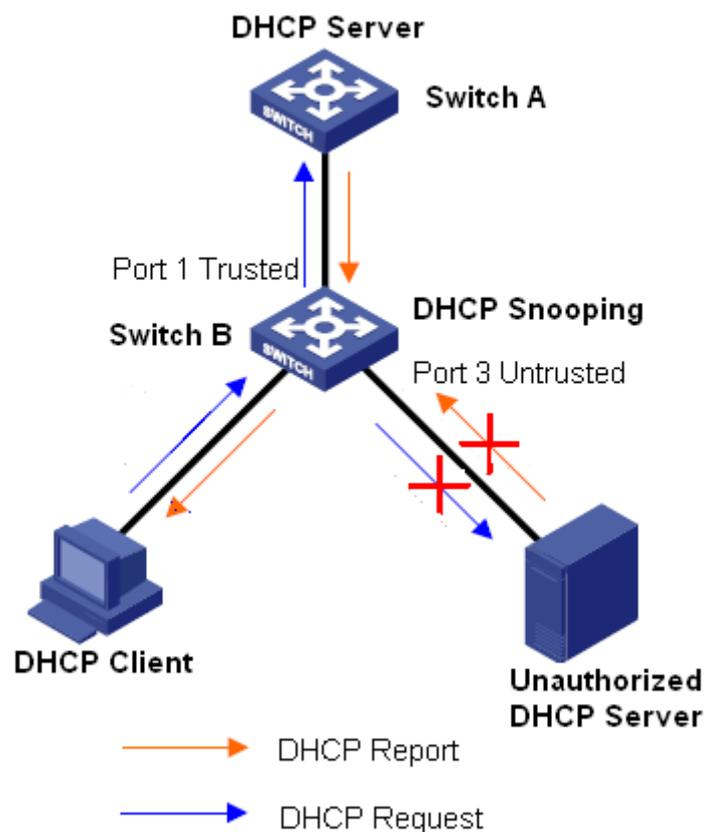
Figure 194 DHCP Snooping Typical Configuration Example
