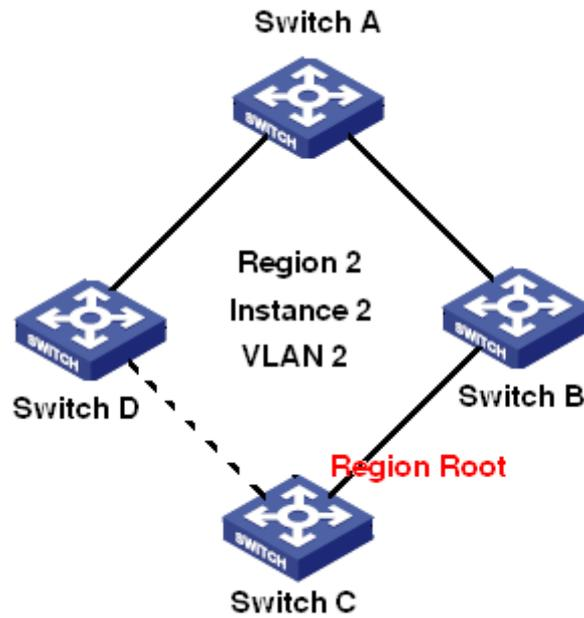
Figure 140 VLAN2 Mapping to Instance 2
