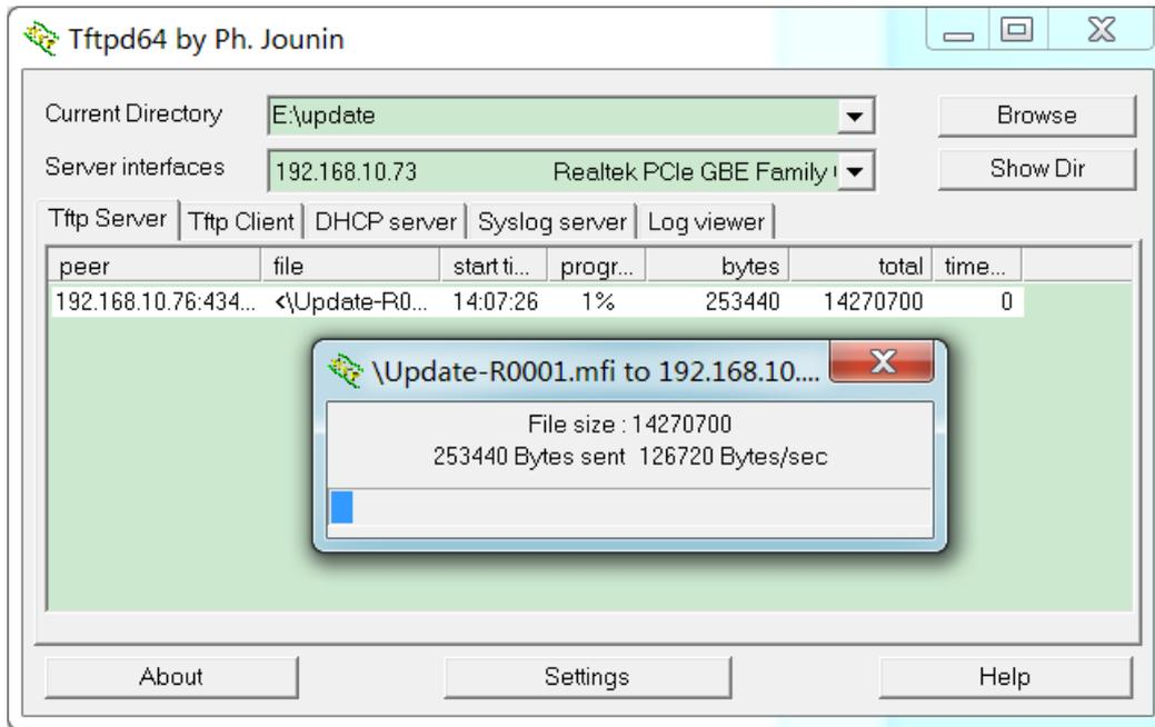
Figure 37 Normal Communication between TFTP Server and Switch
