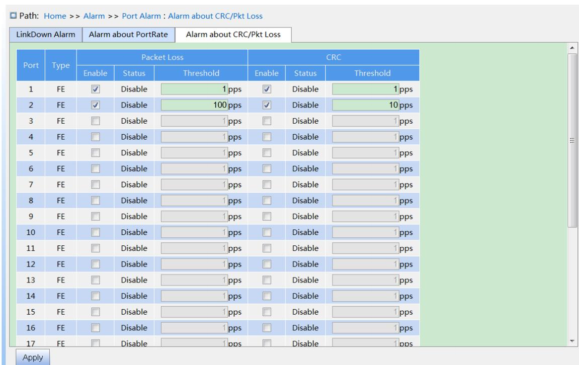
Figure 89 CRC Error/ Pkt Loss Alarm Configuration
