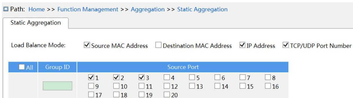
Figure 116 Static Aggregation Configuration
