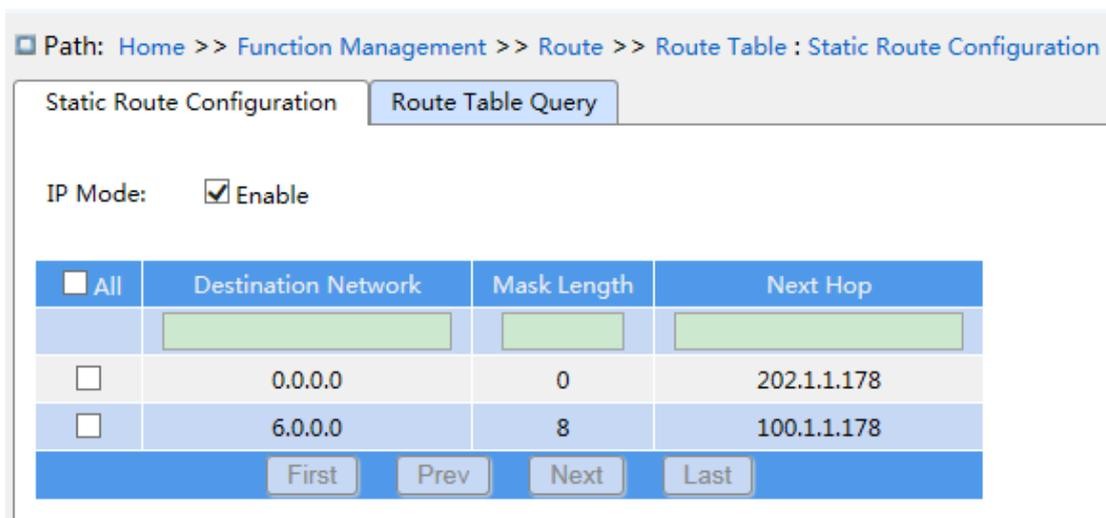
Figure 235 Static routing configuration
