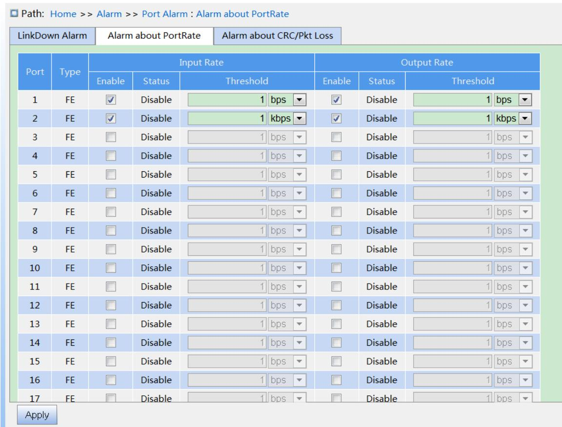
Figure 88 Port Traffic Alarm Configuration
