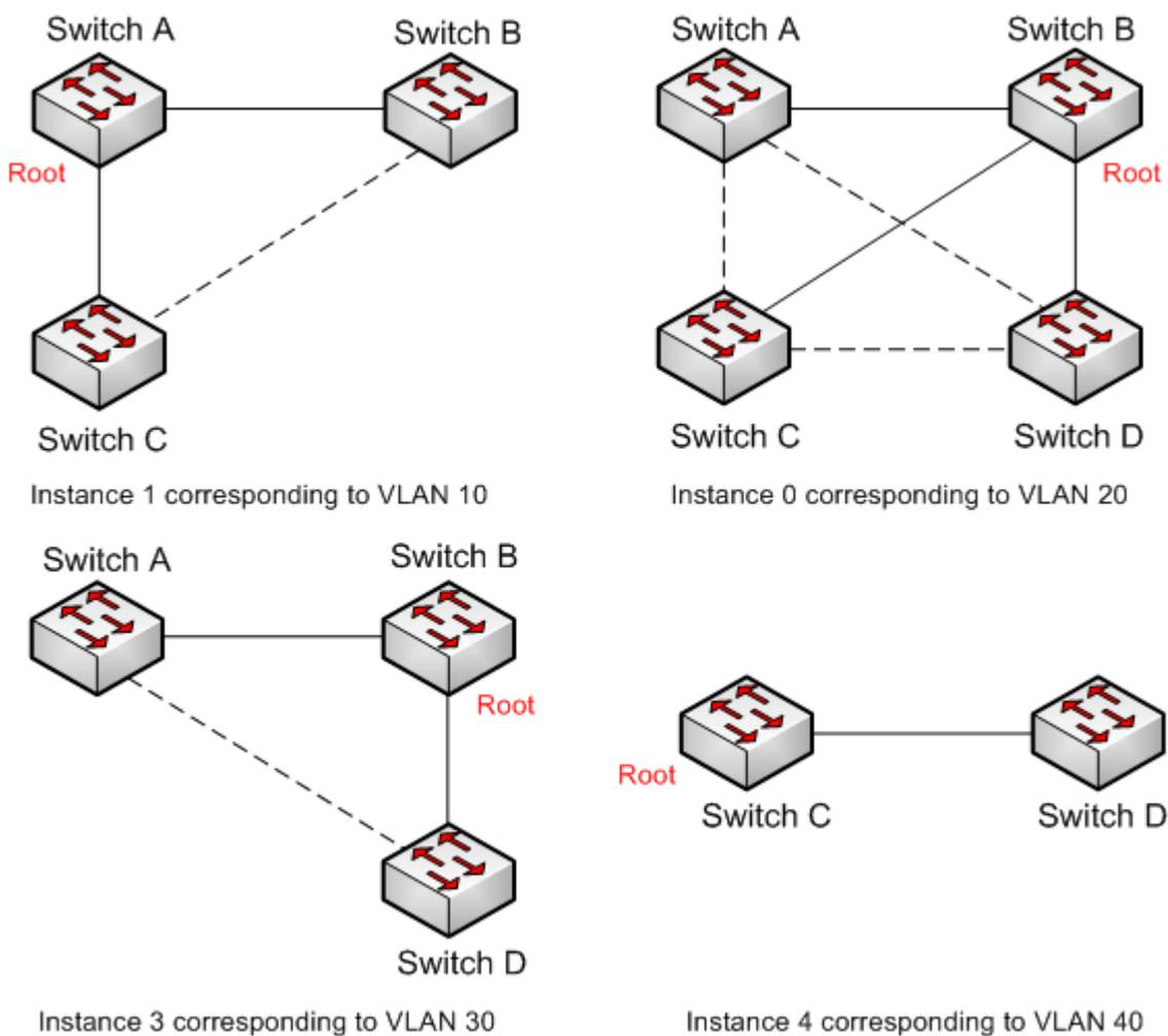
.....Blocked link through MSTP calculation
