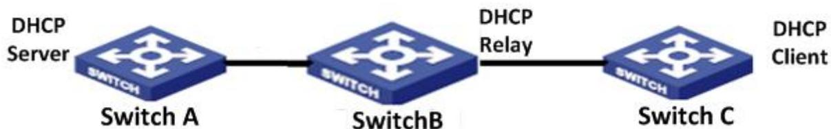
Figure 198 DHCP typical configuration example
