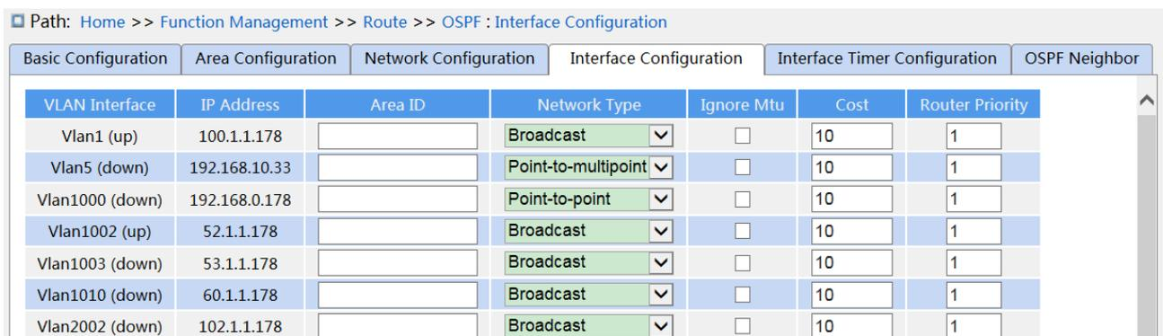
Figure 252 Configure the area and parameters of the VLAN interface
