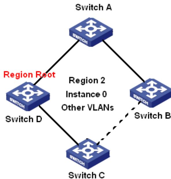
Figure 141 Other VLAN Mapping to Instance 0
