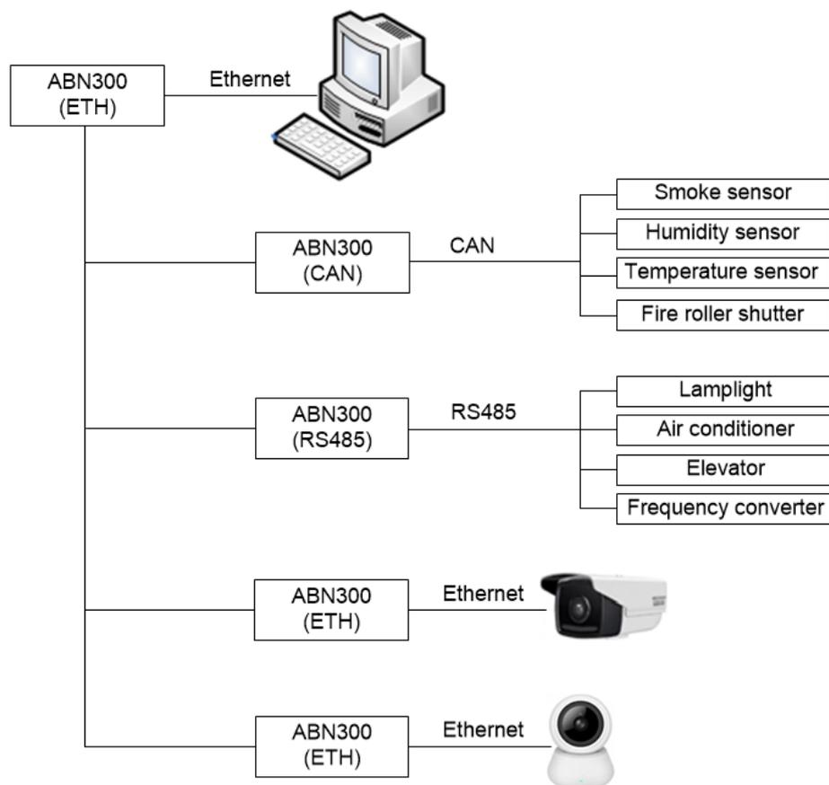
Figure 1 Bus-type AUTBUS Network
